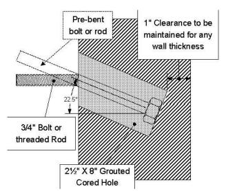
Detail E.1 – Grouted 22½° Inclined Anchor Limitations 22½° grouted anchors shall not be installed with inclination upwards or sideways.
