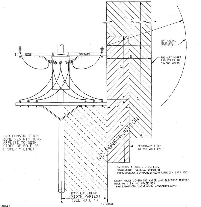
1. OBTAIN APPROVAL IN ADVANCE FROM THE DEPARTMENT OF WATER AND POWER FOR CONSTRUCTION, BOTH PERMANENT AND TEMPORARY, (I.E.SCAFFOLDING, CRANES, PATIOS, STRUCTURES, POOLS, SPAS, ETC) WITHIN THE SHADED OR RADIAL CLEARANCE DESCRIBED ABOVE IN PROXIMITY TO POLES AND OVERHEAD WIRES.
